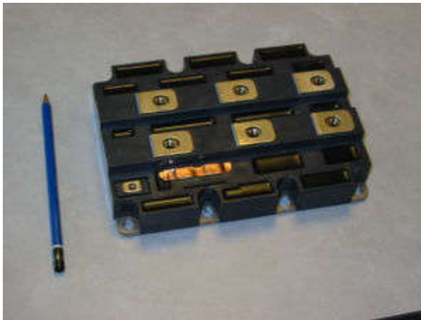
A power IGBT (3300 V/1200 A)
